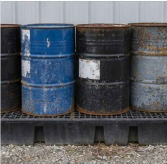
Photo 2: Drum storage on a containment pallet.
