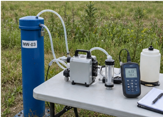
Photo 3: Groundwater sampling setup at MW-03.
